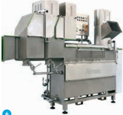
FT15DT Continuous stretcher Output up to 1500 kg/h
