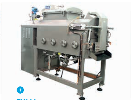
FV900 Steam stretcher Output up to 900 kg/h
