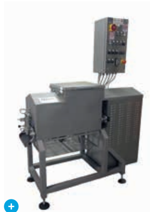
FV100 Steam stretcher Output up to 100 kg/h
