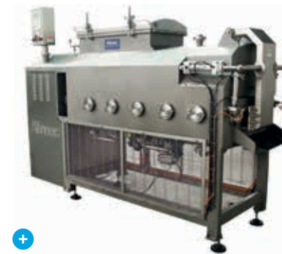
FV1500 Steam stretcher Output up to 1500 kg/h
