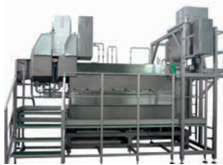
FT30DT Continuous stretcher Output up to 3000 kg/h
