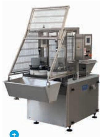
FPB Caciocavallo molder Output up to 1000 kg/h
