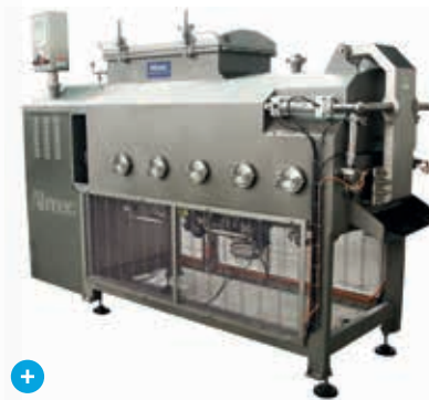
FV1200 Steam stretcher Output up to 1200 kg/h
