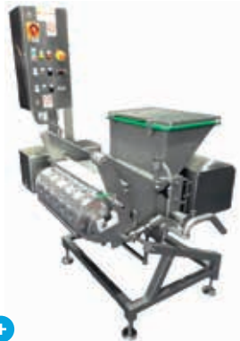
FS100/N Molder Output up to 1500 kg/h
